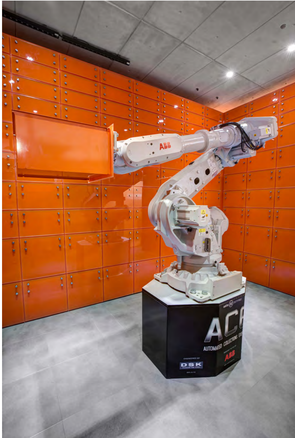
The 'Automated Collection Experience' (ACE) is a click and collect robot at Aelia Duty Free in Auckland which stores your purchases ready for collection when you land. The robot arm opens your secure locker and deposits the purchase in the tray. A fun way of creating interest in an otherwise mundane transaction.
